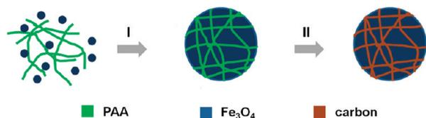
**Figure 1.** Schematic illustration of the formation of the carbon matrix-supported uniform Fe<sub>3</sub>O<sub>4</sub> nanospheres. I: formation of the PAA-entangled Fe<sub>3</sub>O<sub>4</sub> nanospheres. II: carbonization of PAA into carbon matrix.
